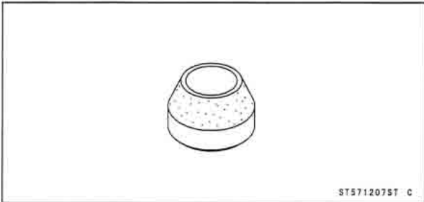
Valve Seat Cutter, 67.5° - \phi 22: 57001-1207
